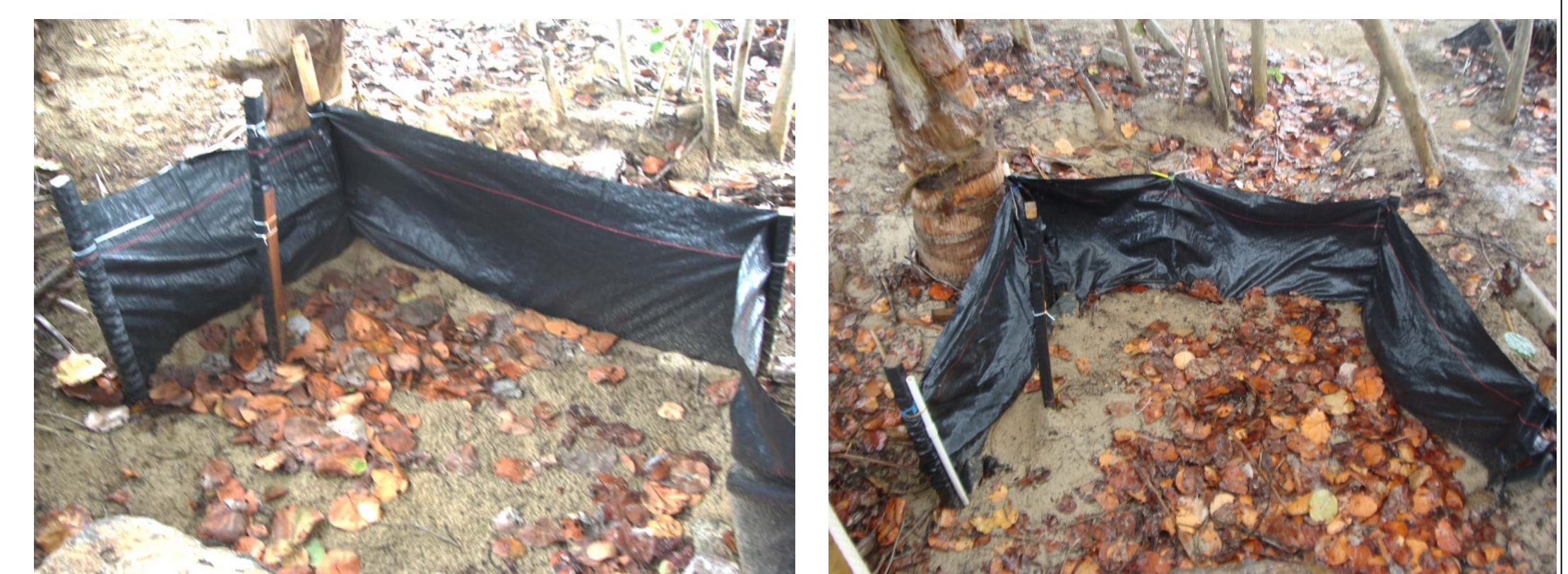
Figure 2. Sediment trap at Zoni initially and after 11 months
