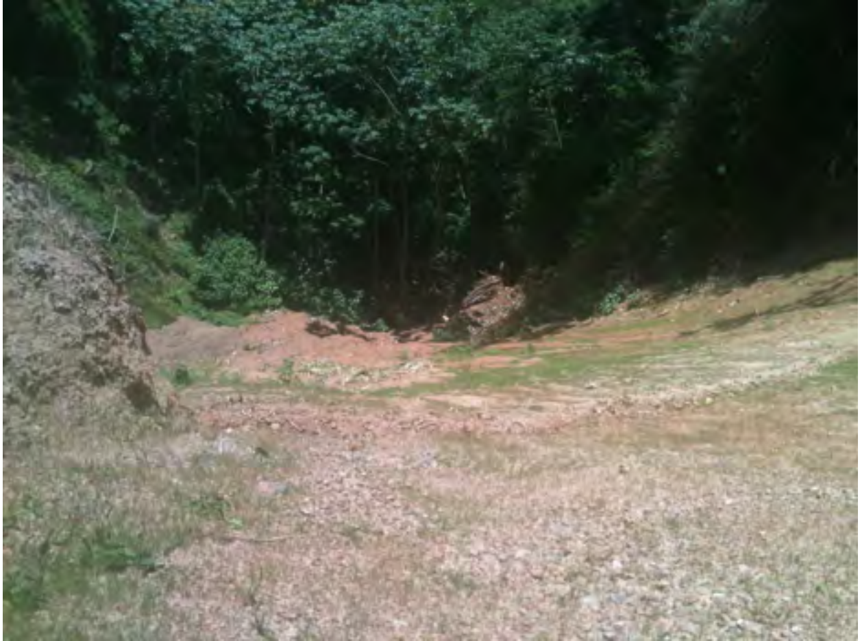
Figure 7. Closeup of Plot 3 -- Thinner application of Flexterra BFM. Note good germination but less vigorous grass growth and the presence of rock
